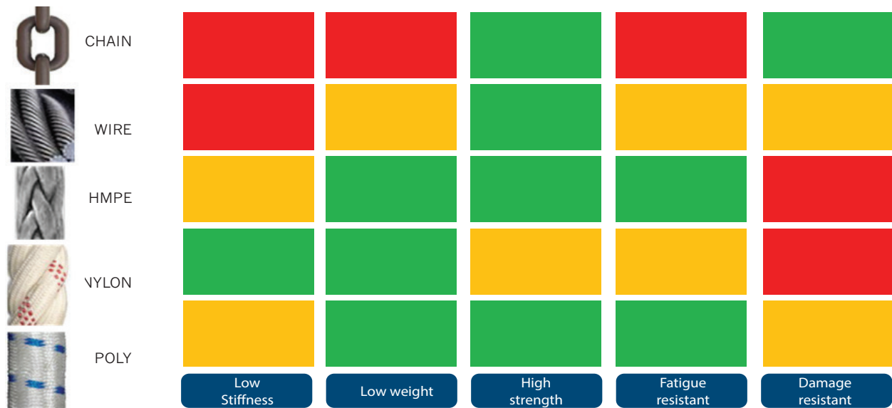
FIGURE 5.3: Guidance on material selection for mooring lines
